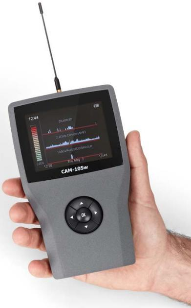
A simple, intuitive menu driven system displayed on a colour TFT screen allows the user to perform real time detection or to view events that have previously occurred. Each band has an individual 20 element signal strength meter enabling the precise source of a detected signal to be located with ease. An audible 'Beep' mode allows the user to monitor without looking at the display and a silent vibrate mode can also be used for particularly sensitive areas.
